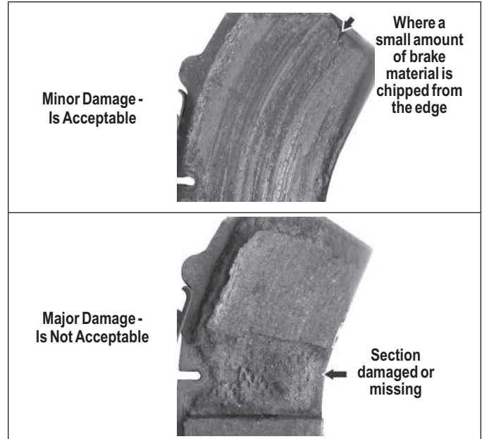
Figure 24 – Brake Pad Surface Inspection
