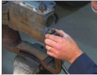
Figure 78 – Position the New Bushing
