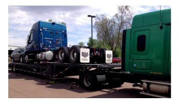
Based off our versatile Next Generation Lo Pro, this modified version is ideal for moving only high profile vehicles. With a tilt deck in the second position you can adjust for a mixed load or for weight distribution. This set-up works well with a Road Tractor with a cab to kingpin distance of 60"-80".
