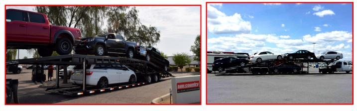
This versatile 5 car hauler is the perfect choice when you have both regional and national transport needs. The lower deck is 20', providing plenty of flexibility to carry trucks and longer-profile vehicles, as well as other various motorized vehicles. A medium duty truck or single-axle tractor is a great fit for this car hauler.
