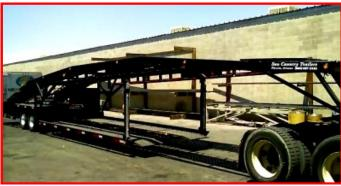
This versatile 4 car hauler is the perfect choice when you have both regional and national transport needs. The lower deck is 20', providing plenty of flexibility to carry trucks and longer-profile vehicles, as well as other various motorized vehicles. A medium duty truck or single-axle tractor is a great fit for this car hauler.
