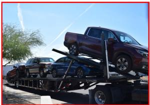
The Sun Country Trailers Air Ride/Air Brake 4 - Car Hauler is our original Road Tractor car carrier. With 53' of useable space it became popular for clients who haul high profile vehicles, and the ability to dump air while loading and unloading helps as well. With the addition of a hydraulic Lift & Tilt deck in the front, this becomes a more versatile trailer with 4 true positions to haul a mixed load.
